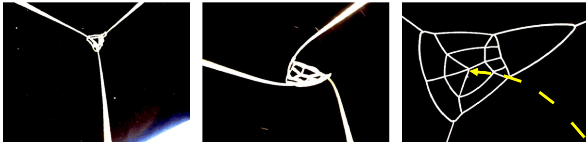
Figure 7: Net spin-up as viewed from the net manager, with desired payload trajectory shown in frame 3
