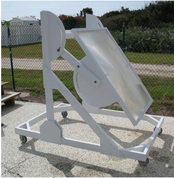
Fig. 2. The 1 m 2 solar concentrator built at NASA KSC.
