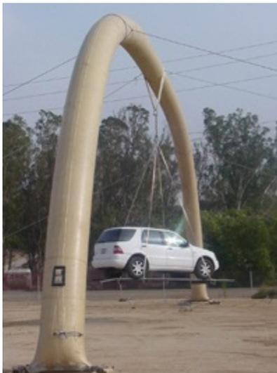
Figure 6. Airbeam supporting a car
