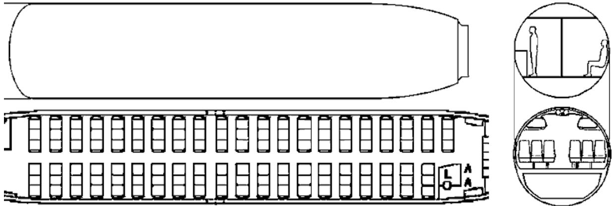
Figure 5. A 3.6x17m cabin compared to a 737-600 cabin
