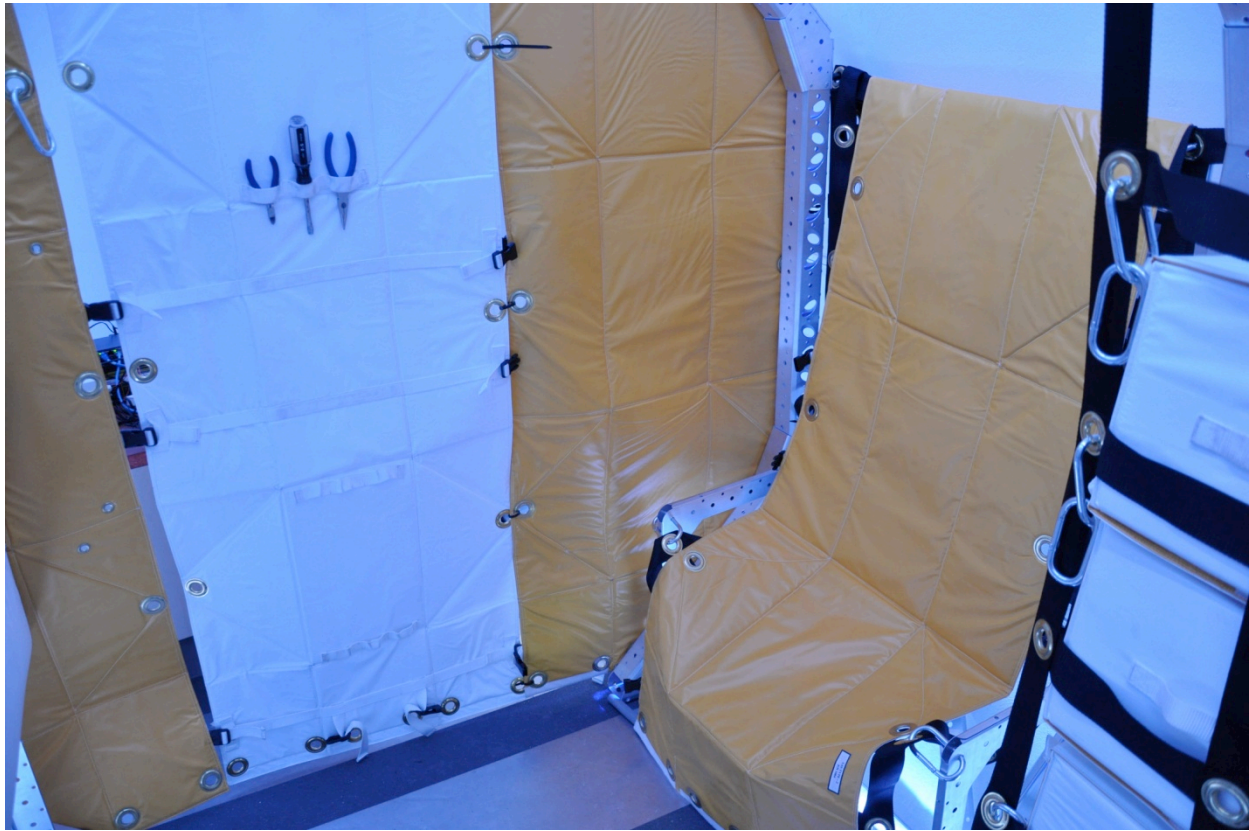
Figure 28 Unfolded CTBs incorporated into wall elements (LSSP Habitation Team).
