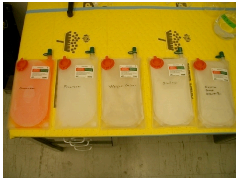
Figure 3 FO flux test run in progress for evaluating four different liquid food products as the osmotic agent and seawater as source water in the LWC-WRS application.
