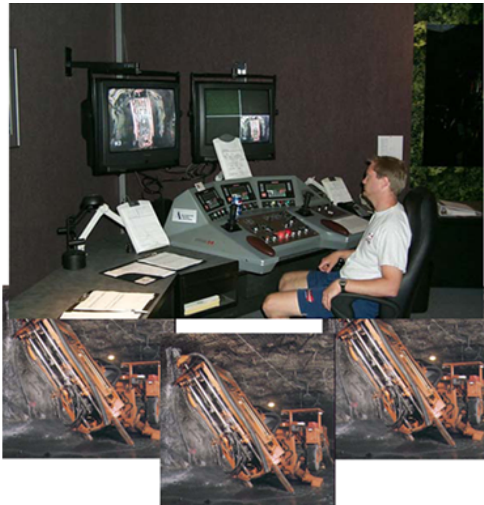
Figure 3 – Teleoperation Control Chair to teleoperate multiple Load-Haul-Dump mining machines from an Operations Centre (courtesy Dr. Greg Baiden)
