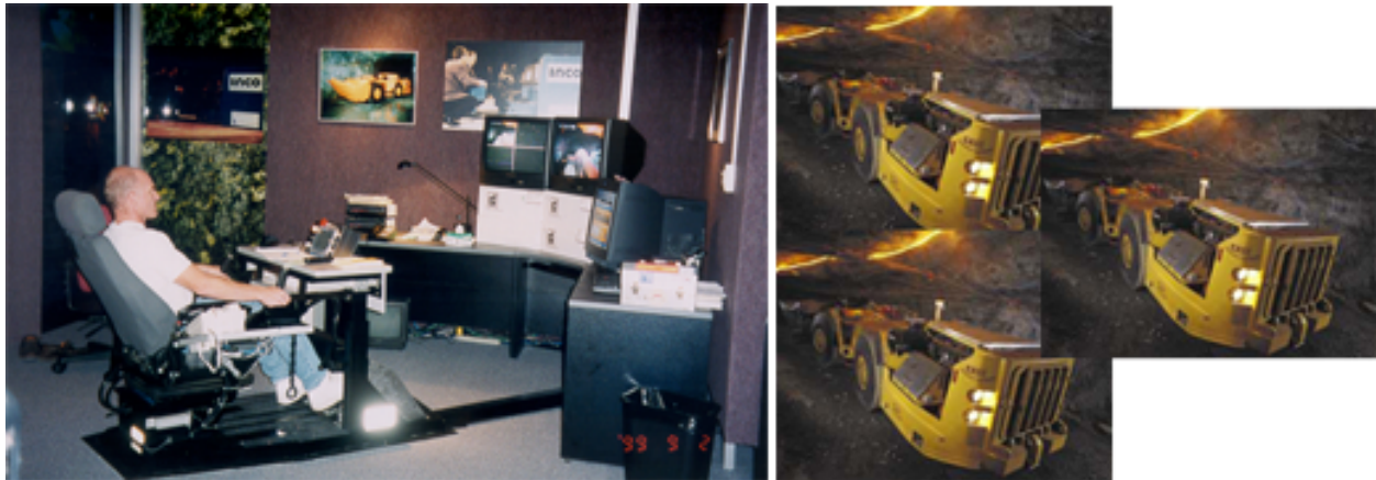
Figure 3 – Teleoperation Control Chair to teleoperate multiple Load-Haul-Dump mining machines from an Operations Centre (courtesy Dr. Greg Baiden)
